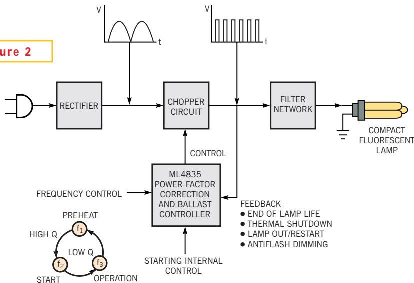
**The compact-fluorescent-lamp controller must provide different functions in the three key cycles of the lamp's operation; it can also provide advanced end-of-life, thermal-shutdown, and dimming functions, all matched to the bulb type.**
