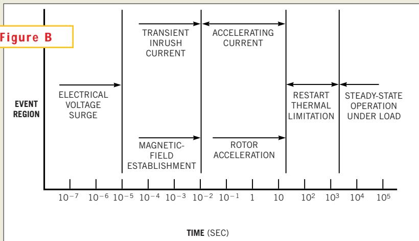
Induction motors go through several critical phases of varying lengths from start-up through steady-state operation (adapted from Reference A).
