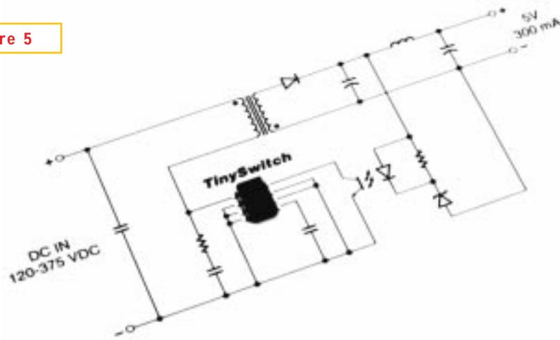
**Using the Tinyswitch from Power Integrations as the core, you can build a wall adapter/recharger that is smaller, lighter, and far more efficient than traditional designs, especially in the common but highly wasteful no- or low-load modes.**
