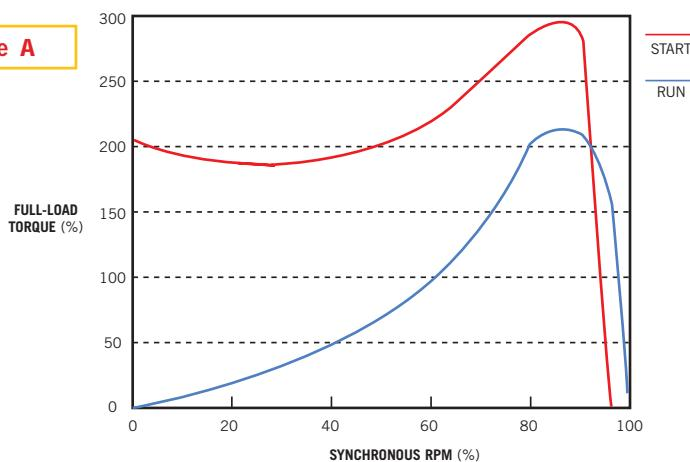
The torque-versus-speed curve for a typical single-phase induction motor shows the rapid falloff in torque outside the 80 to 90% synchronous-speed band (adapted from Reference A).
